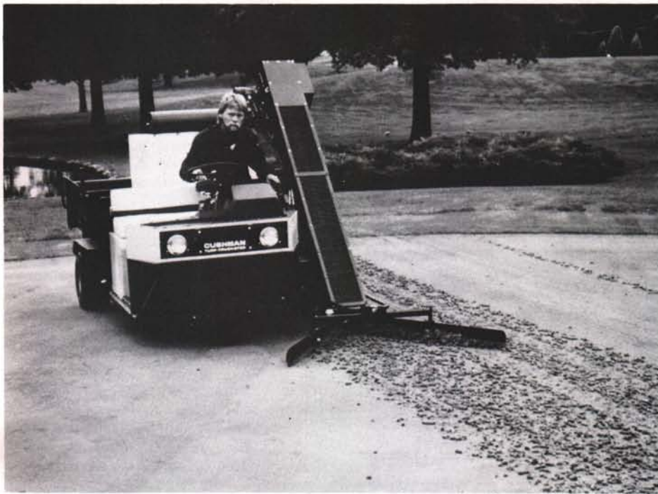
Cushman Core Harvester can clear an average green in 15 to 20 minutes.
