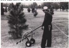
Sports turf managers using FMC's walking boom can accurately spray up to an 80-inch swath of fertilizers or pesticides in compaction-prone turf areas. Connected to a spray unit by a hose, the walking boom provides the precise spray coverage of a boom sprayer without the weight of the tank, pump or turf vehicle.
