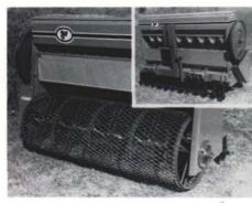
The importance of overseeding to the density and condition of heavily-used sports turf is rapidly gaining recognition. The Tye landscape seeder can do the job quickly and provide a high percentage of seed germination. 42 sportsTURF
