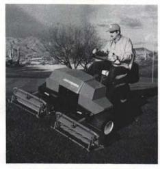
The Tri-King 1471 riding reel mower has been designed by Jacobsen engineers to provide efficient mowing of formal turf areas in an economical machine. A hydrostatic drive system and rear-wheel steering give the Tri-King maneuverability while three 26inch free-floating reels impart a quality cut down to 3/8-inch. The reels automatically stop when the operator raises them with a foot-actuated hydraulic lift—and automatically start again when lowered.
