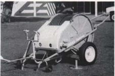
Almost any water source can be used by the Bauer Rainboy to irrigate more than two acres in a single setting. The sprinkler stand and the necessary length of hose are easily unwound from the reel trailer. As the unit operates, the hose pulls the sprinkler back to the reel. After completing a strip up to 500 feet long and 200 feet wide, it shuts off automatically.
