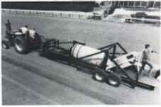
As the value of racing horses goes up, so does the importance of rock-free race tracks, training tracks and exercise areas. One rock hidden in the track dirt can cause a valuable horse to become lame. The Harley Track Sanitizer can remove the threat of a rock injury from a typical one-mile-long dirt track in under six hours.
