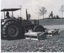
Deutz-Allis has increased the versatility of its 6265 tractor with a Twin-Power PTO option and flail mower attachments. By driving a single front-mounted flail unit with the front power take-off and two belly-mounted units with the rear PTO, the 65 hp tractor can mow a swath 18.5 feet wide.
