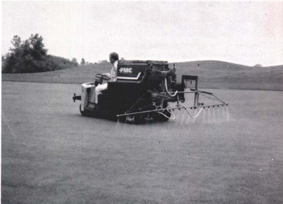
A small truckster-mounted sprayer is used to treat the greens, tees and approaches weekly.
