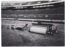
When thousands of dollars ride on a game or race, a rainout is about the worst thing that can happen. After a downpour, standard drainage systems may still take hours to remove excess water from an area. For those who can't wait for hours, a rolling water-remover called the Whale Super Sop-
