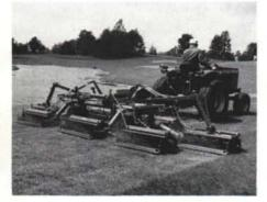
Large-area mowing can still be economical with Brouwer's PTO gang mowers. These transportable mowers can be pulled with small tractors with lower fuel consumption and less weight to cause compaction. The reel units can be lifted for transport manually or with an optional hydraulic lift.
