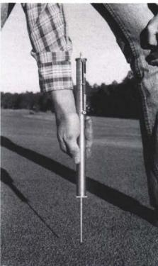
Most sports turf managers have a good idea which areas suffer the most from surface compaction. The Penetrometer can confirm or deny compaction information quickly and enable the turf manager to identify and correct compaction problems before they become serious.
