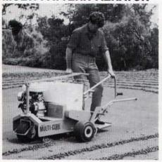
Hole spacing and depth are adjustable on the Multi-Core aerator by S.J. Banks & Son. Three tine heads, one slicer head and one spiker head can be interchanged to obtain the particular type of cultivation needed for all types of greens.
