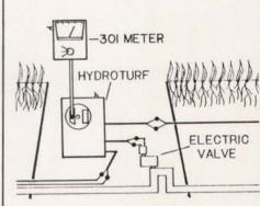
The Hydroturf moisture control system gives the turf manager the ability to automatically override controller instructions to open valves in areas where the soil is sufficiently moist. The system consists of a soil moisture sensor buried in the rootzone combined with a controller and hand-held meter.
