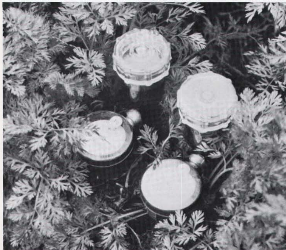
Typical moisture sensing "location." One "short" and one "longer" probe to monitor both the shallow and deep portions of the root system.
