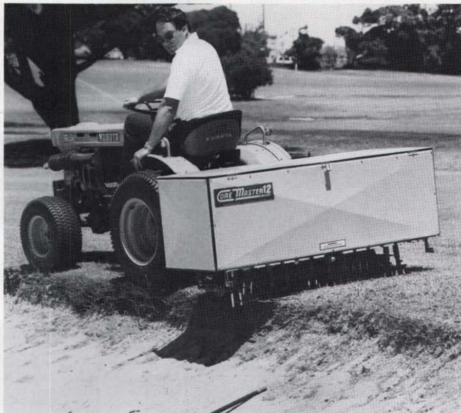
Livingstone demonstrates the stability of his PTO-powered aerifier on the edge of a sand trap.
