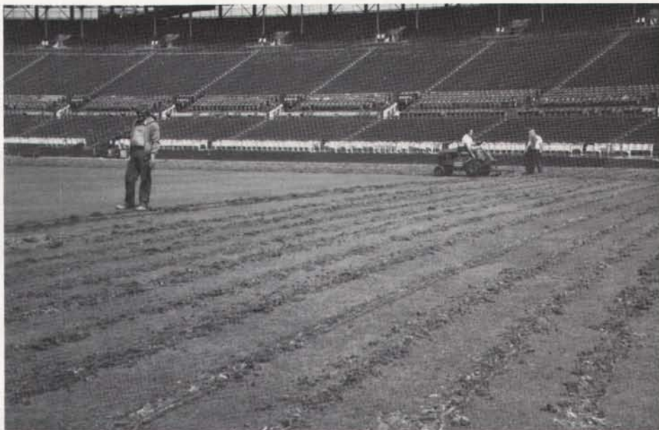
The Verti-Groove cuts and removes narrow, six-inch-deep slices of soil. These slices are removed or broken up with a drag.
