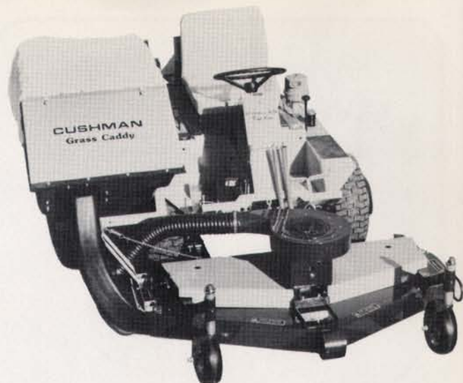
An air-injection system helps Cushman's Front Line rotary pick up wet clippings.
