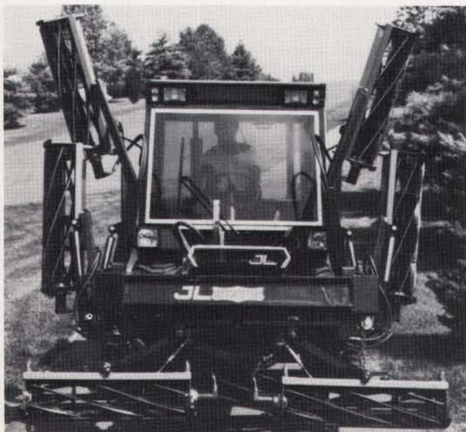
Bunton's Multi-Trac cuts a 16-foot swath but is only eight-feet-wide during transport.
