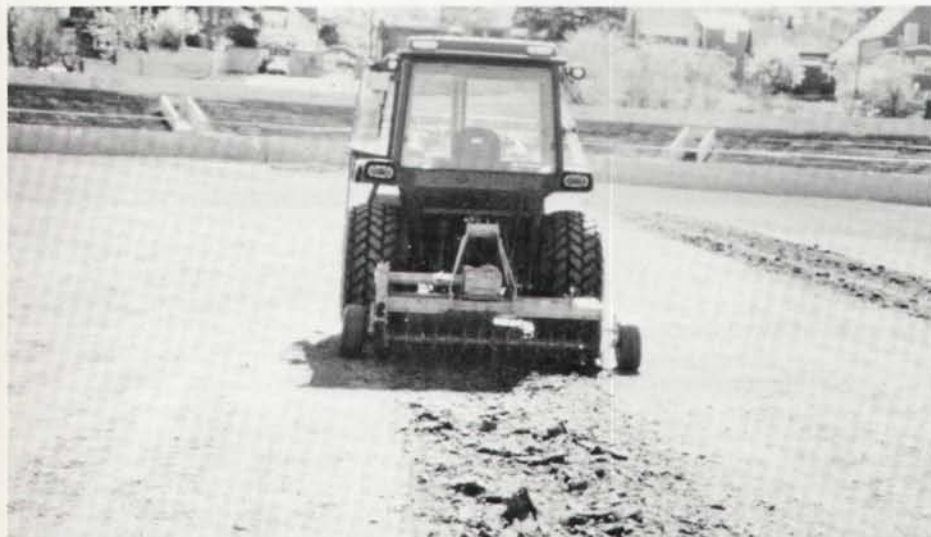
A rototiller with vertical blades breaks up the compacted topsoil.
