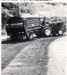
Uniformly spread up to one inch of any topdressing with the large capacity Turf-Topper from Bannerman Ltd. Powered by a tractor PTO, the unit spreads any combination of sand, loam, peat moss, manure or fertilizer through a floor conveyer and contra-rotating spreader cylinder. The unit holds three cubic yards of material fully loaded. Large flotation tires protect turf from compaction or tire damage.
