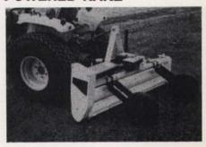
Smaller tractors with 15 or more horsepower can operate Glenmac's five-foot double roller landscape rake. The PTO-driven unit pulverizes seed beds or base paths as it removes rocks, roots, and trash. The result is a soft open surface free of stones and debris. All debris is windrowed by the rake for easy removal.
