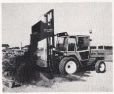
Available in large and mid-size models, Bunton's Multi-Trac multi-purpose maintenance tractors are powered in a choice of 52 hp or 22 hp water-cooled diesel engines. The Multi-Tracs feature a quick connect/disconnect system that allows changing of front-mounted implements in minutes, without tools.
