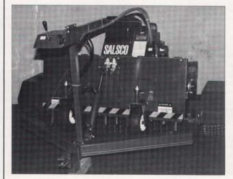
This is a commercial piece of equipment, constructed of 4" Steel square tubing and 34" Steel plate. We have taken our Model 30-12 Greens Aerater and made it twice as wide and twice as strong. Our FTA-60-24 can be towed by almost any vehicle. It is completely self-contained.
