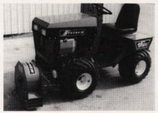
A commercial-grade leaf blower has been added to the list of attachments for the Steiner center-pivot tractors. Heavy steel housing, a 14-inch fan and industrial relube bearings assure long life and extra power for the blower.
