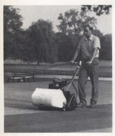
The trend toward faster putting surfaces has been recognized by Jacobsen with the introduction of its ultra-fine-cutting greens mower. Nine-bladed reels are adjustable from 3/32 to 7/16-inch to enable superintendents to cut greens as low and as smoothly as possible. Adjustments are fixed to assure a consistent height of cut.
