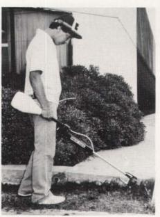
CDA technology allows treatment of large areas with noticeably reduced volumes. According to the manufacturer, one worker with a five-pint Microflex bottle can treat a strip eight inches wide for 20 miles without stopping for a refill.
