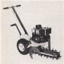
Trenching in confined, small and hardto-reach areas is possible with the Ground Hog Model T-4 Trencher. Powered by a 5 hp gasoline engine, the T-4 digs a trench 3½ inches wide and from six to 12 inches deep below the reach of most turf aerator tines.
