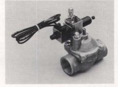
All-brass solenoid control valves have been designed by Griswold Controls for dirty water applications. The valves range in size from 3/4-inch to two-inches and will maintain a constant downstream pressure when upstream pressure varies from 5 to 200 psi.
