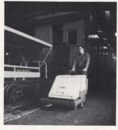
The Tennant Model 186 walk-behind sweeper can clean 18,000 square feet of indoor or outdoor surface an hour, nearly six times faster than hand methods. The unit sweeps a 34-inch path and can be converted to a scrubber in minutes, without tools.
