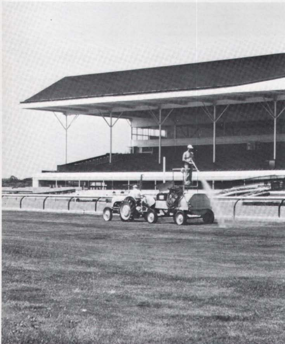
Race track grounds crew applies a surfactant to infield to eliminate dry spots and to obtain uniform turf appearance.
