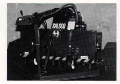
Sports turf managers can aerate at up to 40 holes per square foot with a new commercial trailing aerator from Salsco. The FTA-60-24 is twice as wide as the company's greens aerator cultivating up to a 60-inch wide swath on each pass.
