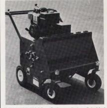
CORE-AERATORS - Self-propelled, walk-behind units which come in these models: 36-6, 30-6, & units which come in these models: 36-6, 30-6, & 30-12. Penetration up to 3" using ¼, ¾6, ½, ¾6 or ¾" tines. Five horsepower Briggs & Stratton IC engines are standard. We offer Honda as an option. Easy maneuverability with coring rate of up to 30,000 sq. ft./per hour. All models weigh under 300 lbs. and give straight in & out holes no tearing of turf.
