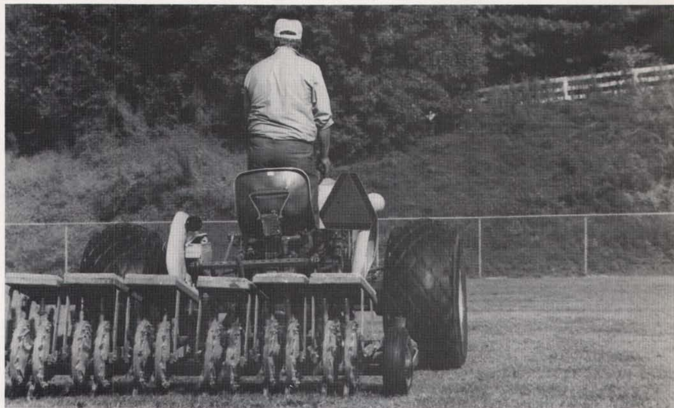
Field (below) is aerated prior to fertilizing to help mix fertilizer into the rootzone.
