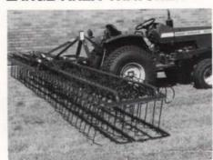
Four thatcher models for large areas are available from Lely. Models range in width from seven to 20 feet while operating, yet measure only seven feet during transport. The number of tines can be tripled to reduce the number of passes and save time. Thatching severity can be adjusted by five tine positions.
