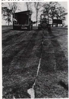
When drainage is insufficient and the season is about to begin, you need a way to open up drainage without severe disruption to the playing surface. A Britishmade sports drainer is now available to do just that.
