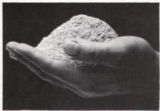
A new clay carrier for Elanco's Balan improves spreadability, reduces dust during application, and increases calibration accuracy. The manufacturer says clay spreads more uniformly than corncob or limestone carriers.
