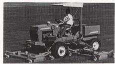
Jacobsen's new HR-15 can cut nearly a 16-foot swath through semi-formal and rough turf with three hydraulically powered 72-inch rotary decks. The decks float in front and on both sides of the tractor providing great maneuverability; they are raised and lowered hydraulically.
