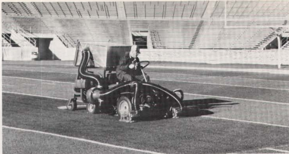
The stadium field is mowed at 7/8-inch three times per week using a Ransomes 230D with vacuum for clippings.
